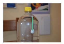
Drop the straw onto the bottle and screw on the top. The diver should be floating at the top of the bottle. Squeeze the bottle and the diver should sink to the bottom.
